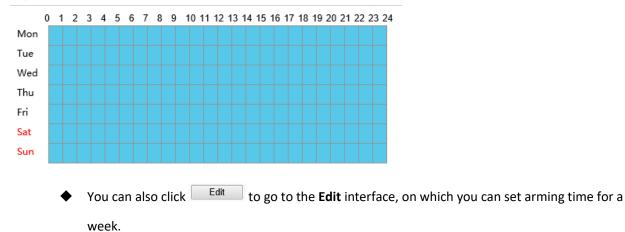
A maximum of eight arming time ranges can be set for a day. The time ranges cannot be overlapped. A recognition success prompt is displayed only when the authentication succeeds in the preset arming time ranges. The prompt "non-specified time" is displayed when the authentication is successful out of the arming time ranges.
